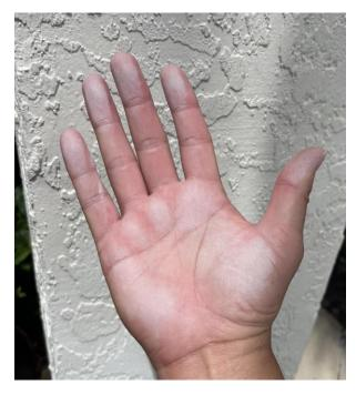
Chalk is present on various surfaces throughout the community. Through cleaning should be done anywhere chalk is present. ALL previously painted stucco should be primed with Loxon Masonry Conditioner (LX03 Series) prior to painting. Additional surfaces where chalk is present should receive a prime coat of conditioner as well.
